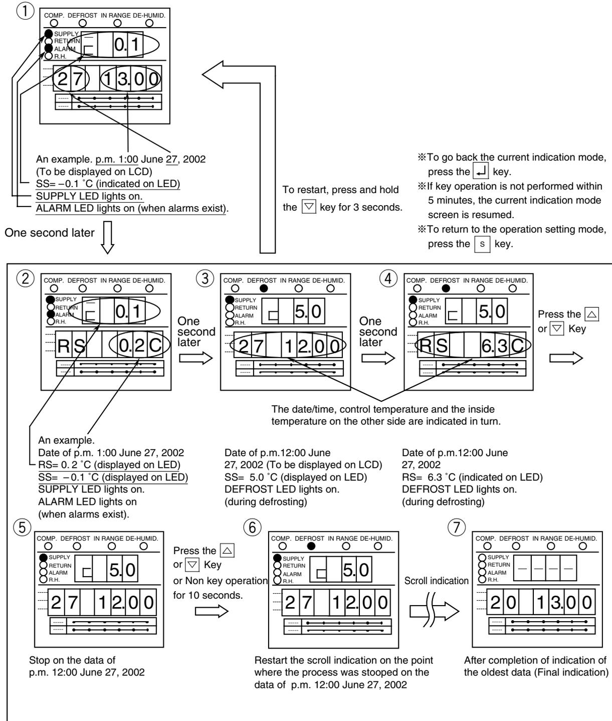
Note: "□" on the leftmost of the LED shows that the indication is of the temperature record scroll indication mode.
