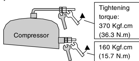
3. Fix the suction and discharge flanges using with the auxiliary gaskets and the bolts.
