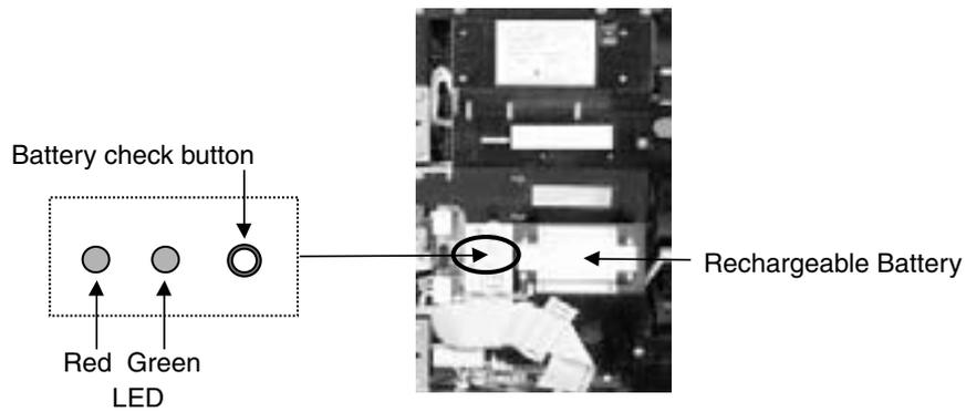
To test residual voltage, check color of LED by pressing battery check button.
