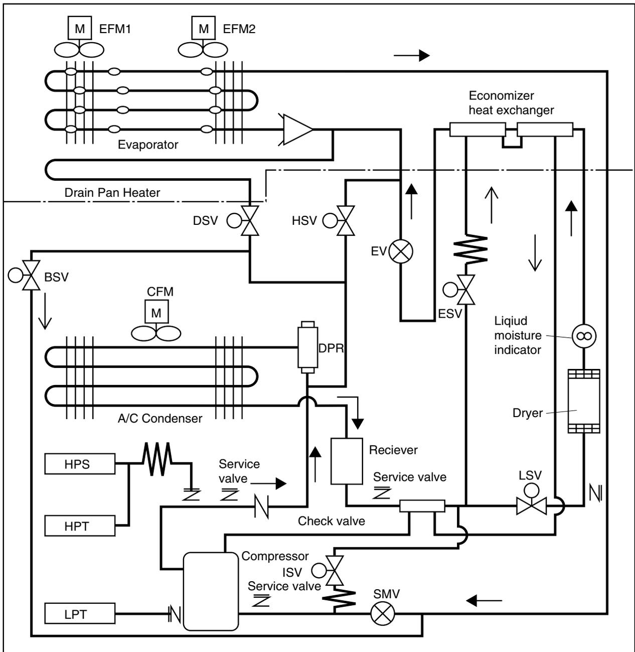
EV :Electronic Expansion Valve    SMV:Suction Modulation Valve    DPR:Discharge pressure regulator
