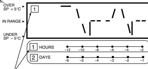
The graphic chart of the temperature change for 12 hours log (time base : 1 (HOURS))
