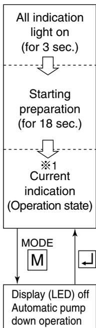
Press the <sup>MODE</sup> **M** key in current indication mode to go to Display (LED) off / Automatic pump down operation.
