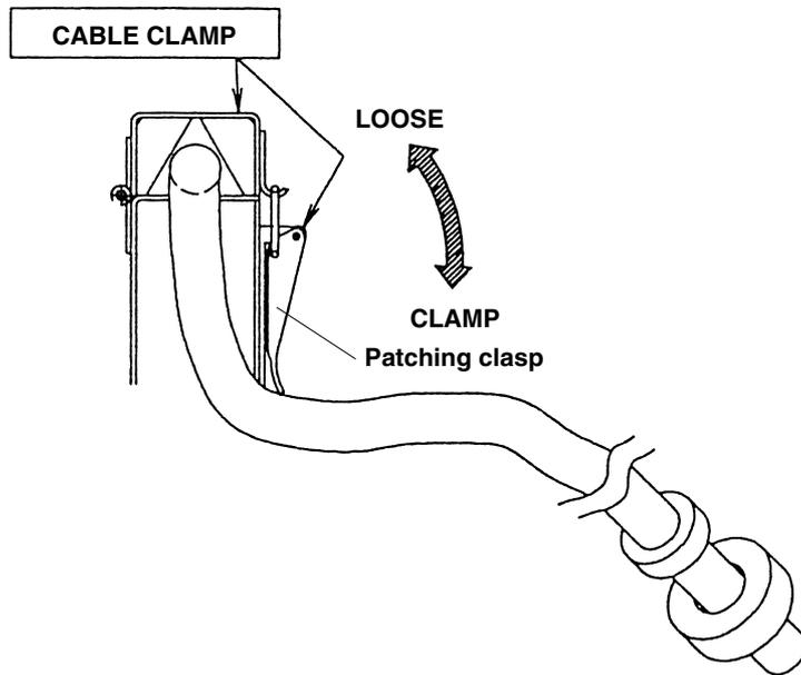
**8.3.3 Cable clamp bracket 2 (Applicable models:LXE10E-A5(BR),A7,A8,A9, A11,A20,A26(A),A12(AtoE),A28,A17(A),A35(A),A19, and A26(B,C))**
