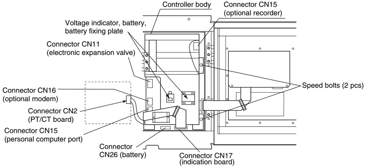
(2) Open the controller body, then disconnect the connectors ② through ⑧ on the terminal board mounting plate ⑩.
