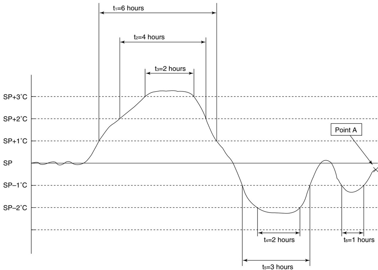
Example : If inside temperature was recorded above graph, controller shows the following "d code" when user check the code at "point A"
