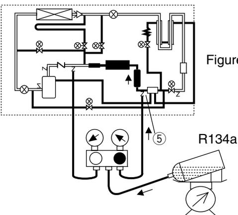
2. Replace the manifold gauge hose to port ③ and add the liquid refrigerant. Then if it reached to the specified amount close the cock of the refrigerant cylinder.
