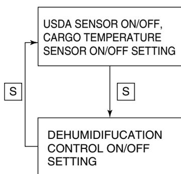
To set the USDA ON/OFF and CARGO TEMPERATURE SENSOR ON/OFF: Select "OFF (not in use)", "3 (3 USDA probes are in use)", or "4 (3 USDA probes and 1 cargo temperature sensor are in use)" on the LED while the LCD displays "USdA".
