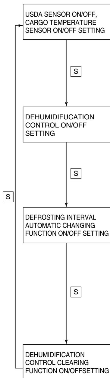
To set the USDA ON/OFF and CARGO TEMPERATURE SENSOR ON/OFF: Select "OFF (not in use)", "3 (3 USDA probes are in use)", or "4 (3 USDA probes and 1 cargo temperature sensor are in use)" on the LED while the LCD displays "USdA".
