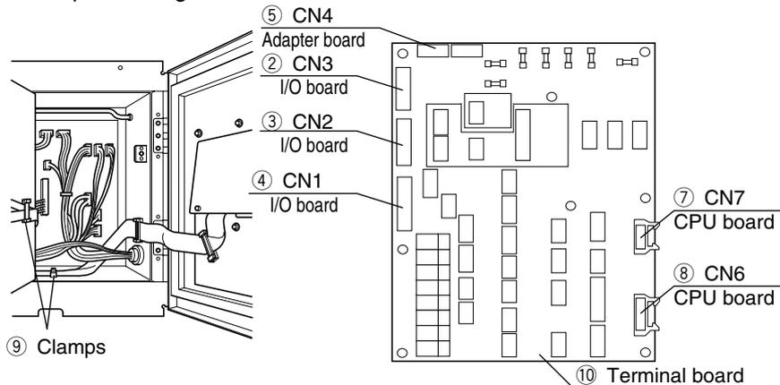
(4) Remove screws (2 pcs) fixing the controller, and replace the controller with a new one.
