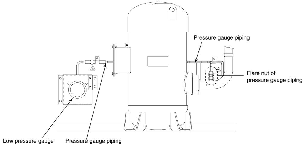
When the flare nut of pressure gauge piping is loosened for replacing pressure gauge, "LOCTITE" and "Sylicone sealant" should be applied by following precedure to prevent refrigerant leakage caused by freeze of moisture.
