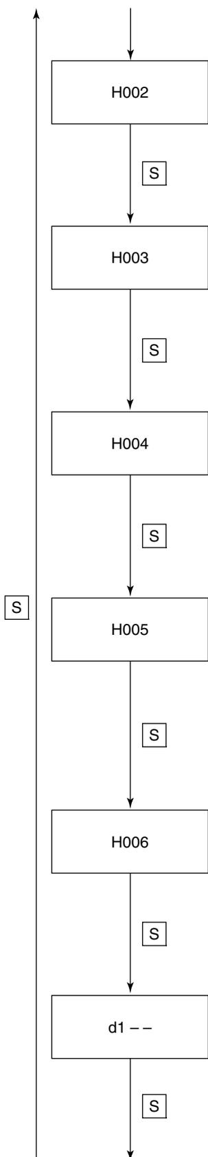
H002 code is displayed when the integrated time of Out-of "In-Range" reaches 2 hours.
