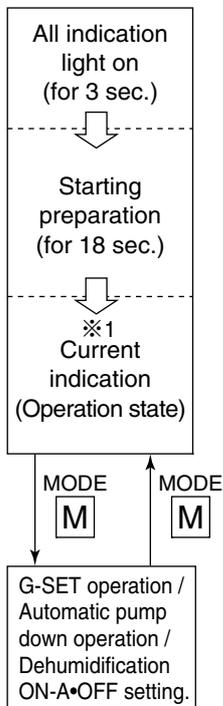
Press the <sup>MODE</sup> **M** key in current indication mode to go to G-SET operation / Automatic pump down operation / Dehumidification ON-A · OFF setting.
