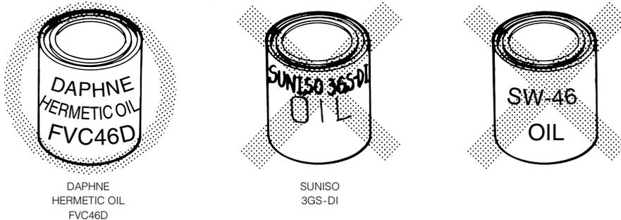
**Open the oil can, just before charging the oil, and use all the oil in the can once opened.**
