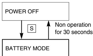
To change to the BATTERY MODE, press the [S] key while the unit is in the POWER OFF STATUS.
