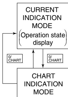
To shift to the chart indication mode, press the
