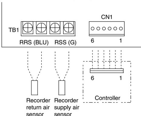
**(3) Checking (Calibration) of the indicated value on the recorder (optional)**
