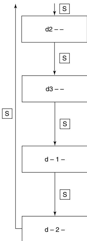
"d2 --" message displays the total time in hours, that the temperature was above set point +2°C. The code will be displayed after the selected time which can be set to: "1"hour, "2"hours, "3"hours, "4"hours, "5"hours, or "10"hours. When the total time above set point +2°C reaches "1"hour, the code "d101" will be displayed.
