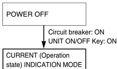
Turn on the circuit breaker and the UNIT ON/OFF key after turning the power supply on, then the display panel switches to the CURRENT INDICATION MODE. (Key operation in the CURRENT INDICATION MODE is possible after approx. 21 seconds from turning on the UNIT ON/OFF key.)
