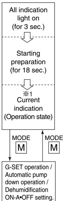
Press the <sup>MODE</sup>
