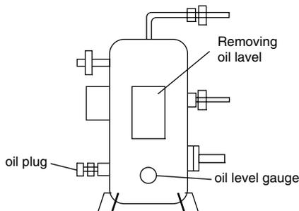
○ When the compressor is replaced to spare parts compressor, remove the excess refrigerant oil in the following procedure.
