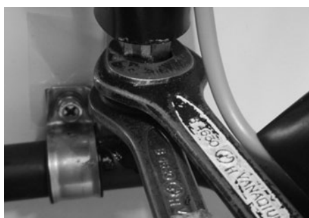
Fig. 1 Use two wrenches when removing and installing.
